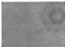
Routine intrinsic uniformity, 99m Tc, 15% energy window, 128 × 128 matrix. The image has been contrast enhanced.
