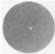
Uniformity image. A discrete circular cold area is seen in the middle of the FOV. Visual inspection of the flood source revealed a large air bubble. The cold indentation at the top left edge of the FOV was also due to an air bubble.
