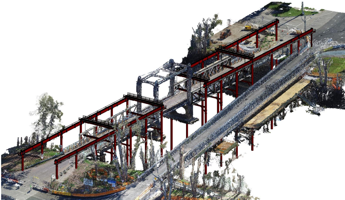
Figure 5.0. Laser scanning of existing bridges with the proposed bridge geometry shown in dark red.
