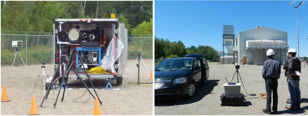
Figure 2: Site installation of INO mobile laboratory, folding mirrors in forefront (left) and view of the compression station (right).
