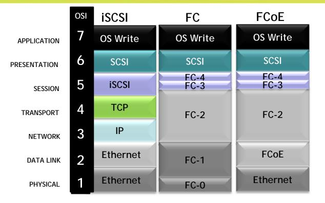
Fibre Channel is a layered protocol. It consists of 5 layers, namely:
