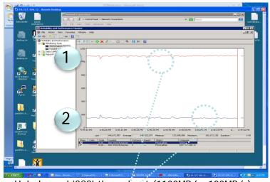
Unbalanced iSCSI throughput (1100MB/s, 100MB/s) Typical TCP burstiness
