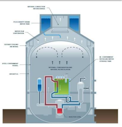
The **AP1000** plant is designed to reduce or eliminate the chances of a core meltdown and explosion in situations where the plant experiences a total loss of power, similar to the accident at Fukushima.
