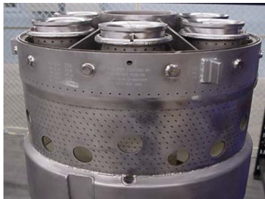
Figure 4. LECIII® Combustion Liner Head End Mixer Effusion Cooling Holes
