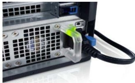
Easy troubleshooting. Functioning PSU handle glows
