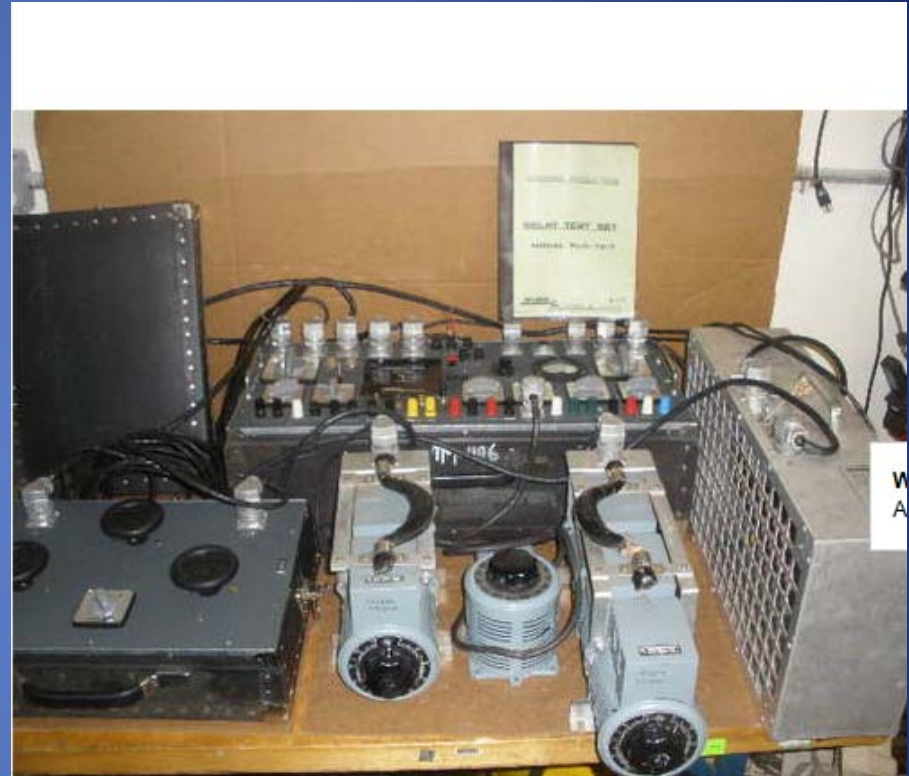
Wilmar three phase set with variacs, phase shifter, load box, and timer.
