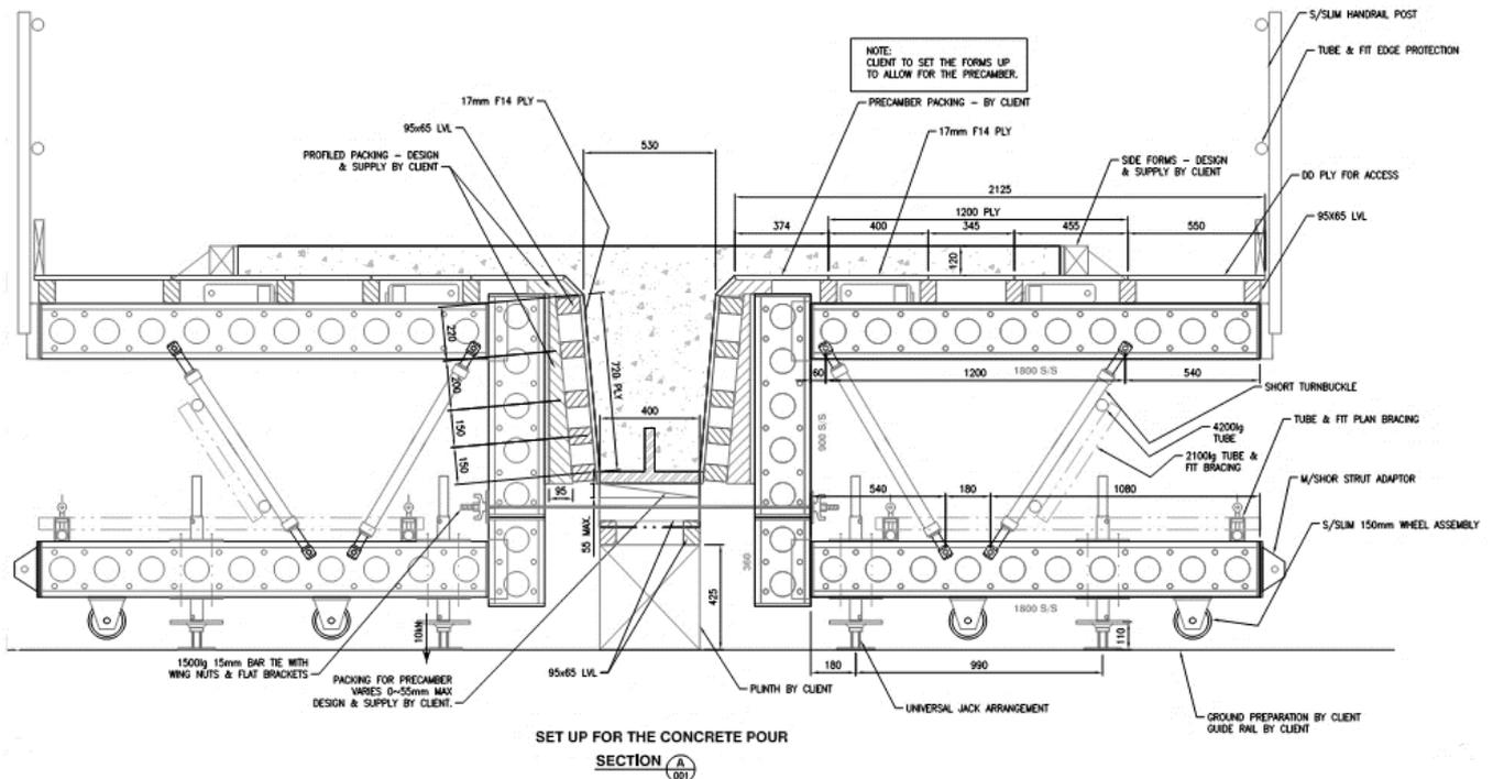
Plate 12: Formwork set-up
