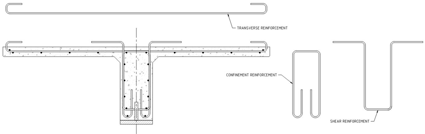
Plate 1: Typical reinforcement for a T-girder with a halved I-girder utilised as external reinforcement
