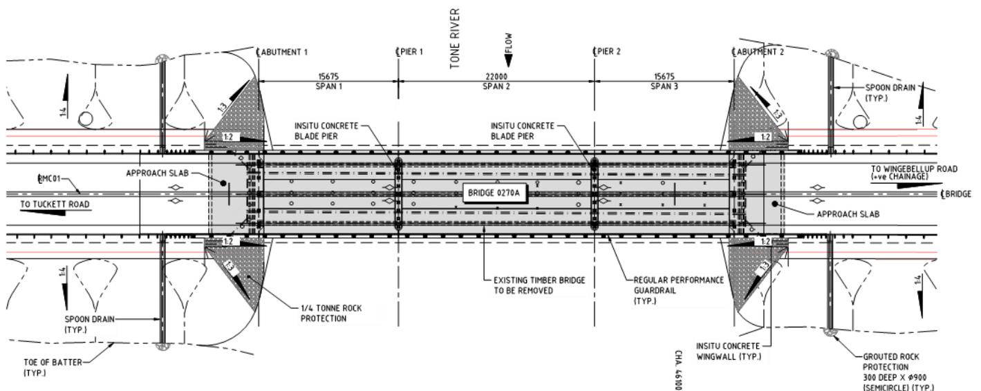
Plate 7: Plan view 3-span arrangement
