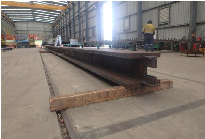
Plate 10: Welded beam before cutting
