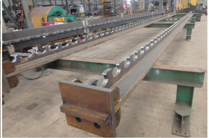
Plate 11: Welded beam after cutting in half, including the end compression plates
