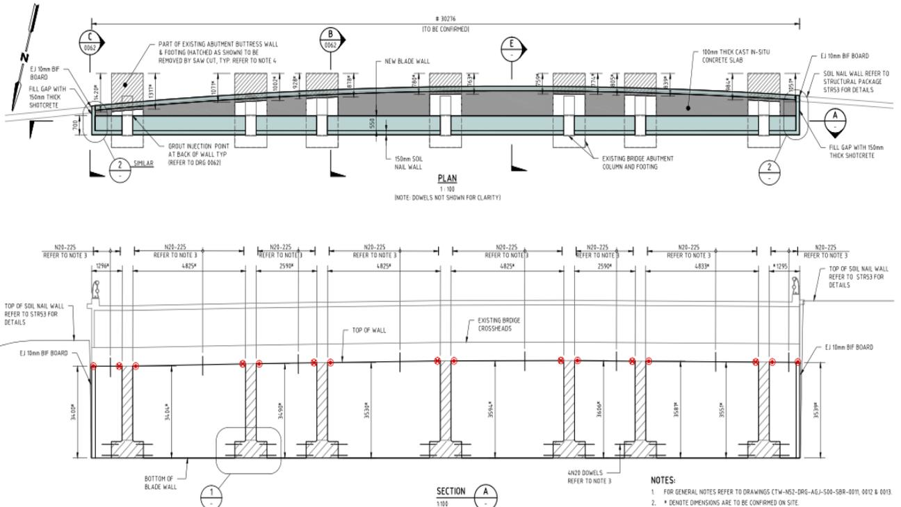
Figure 4 – Detail of Existing Footing Demolition and New Wall
