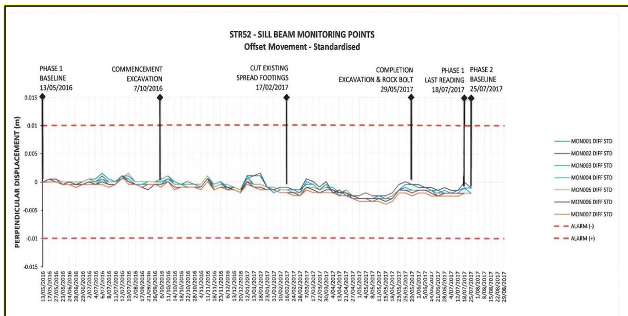
**Figure 8 – Abutment Sill Monitoring Results**
