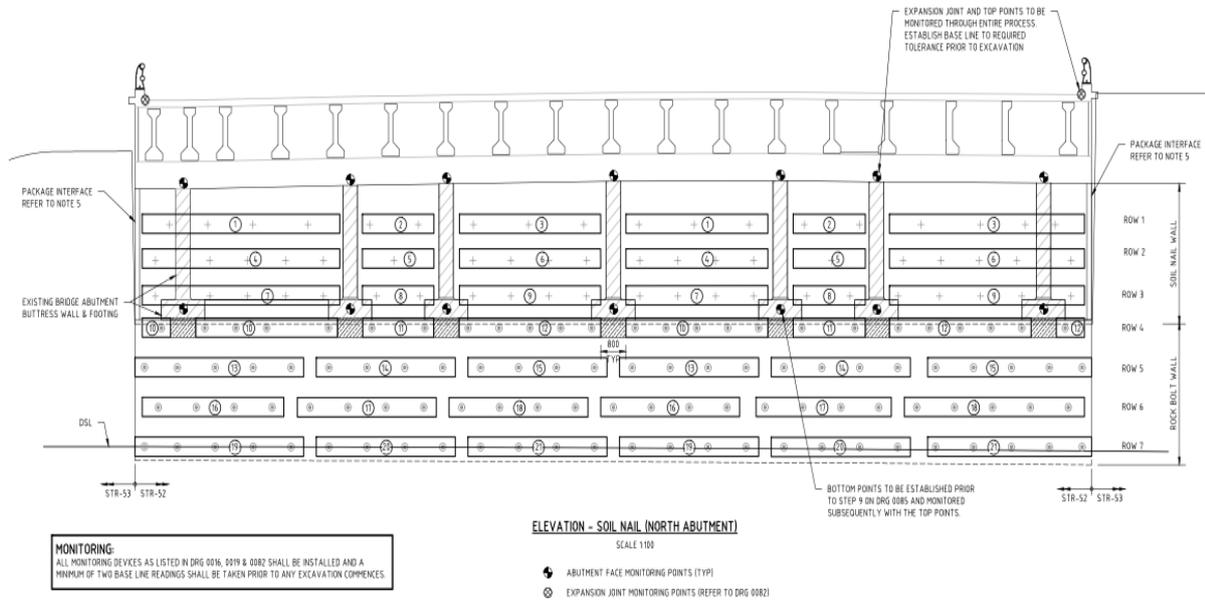
**Figure 7 – Abutment monitoring and Excavation sequencing details**
