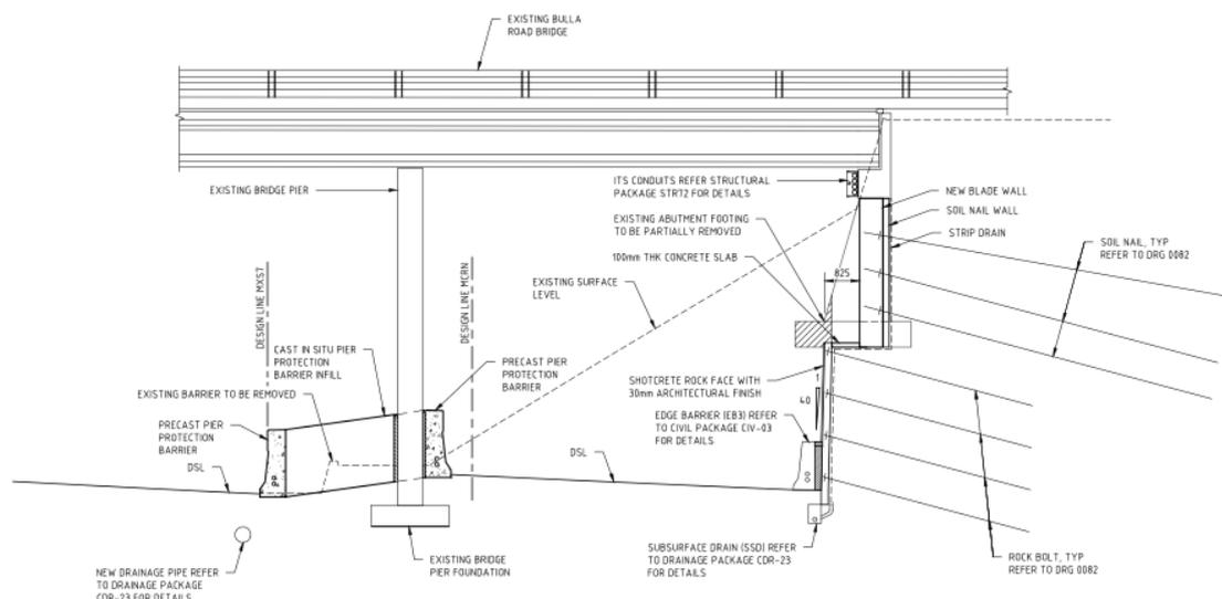
**Figure 3 – Elevation-Abutment Modification**
