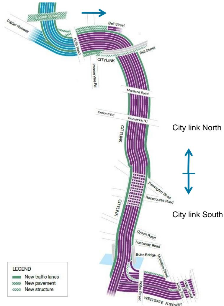
Figure 1 – Schematic CTW Sections
