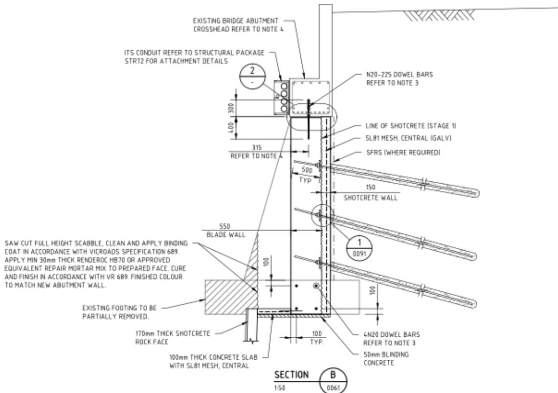
Figure 5 – Detail of New Wall and Soil Retention System
