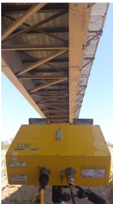
Figure 5. IBIS-FS was set up directly under the bridge to maximize the power of the return signal to the receiver from each range bin
