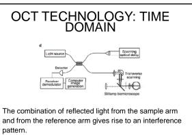
This interference pattern is detected, and the info is processed to produce measurements of magnitude and echo delay time 1
