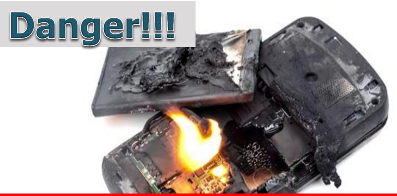
Counterfeit batteries have sub-standard safety features and may be damaged and unsafe
