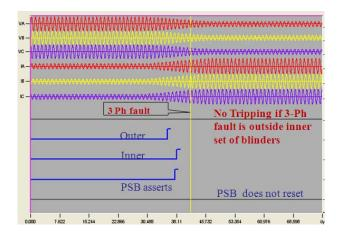
Fig. 40 Oscillograph Showing PSB Assertion and Blocking of Zone 1
