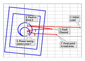
Fig. 34 Test Scenario With Fault and Power Swing
