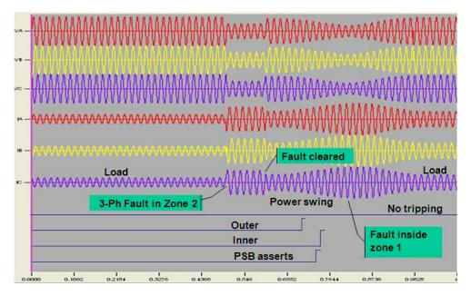
Fig. 36 Plot of Waveforms and Relay Operation
