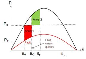
Fig. 3. The Equal-Area Criterion (Figure shows a fast fault clearance and a stable swing)
