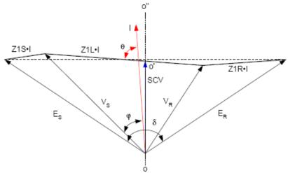
Fig. 18 Voltage Phasor Diagram of a Two-Machine System
