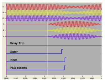
Fig. 27 Voltage and Current Waveforms Seen By Relay
