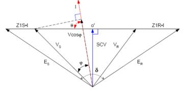
Fig. 19 Vcosp is a Projection of Local Voltage, VS, Onto Local Current, I
