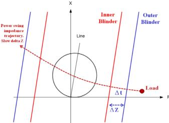
Fig. 9 Two-Blinder Power Swing Detection Scheme
