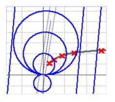
Fig. 39 Power Swing and Fault in Zone1 Outside the Inner Set of Blinders
