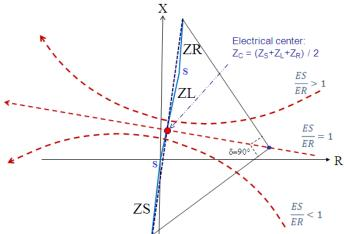
Fig. 6 Impedance Trajectories Seen By a Distance Relay at Bus S
