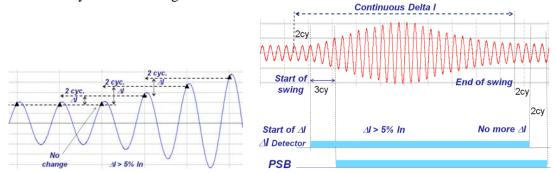
Fig. 14 Continuous Superimposed Current Method
