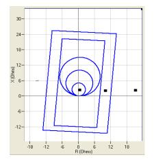
Fig. 21 Graphical User Interface for Entering State Simulation Impedance Points
