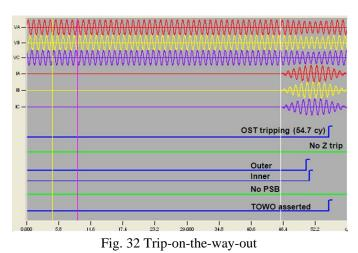
The second case for trip on the way out resulted in tripping at 54.7 cycles from the start of the test, well after the swing leaves 180° going left, as shown in Fig. 32.
