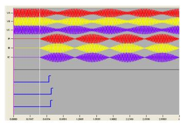
Fig. 29 Simulation of Multiple Pole Slips
