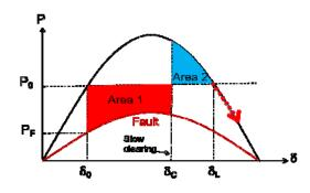
Fig. 4. Unstable System due to Slow Clearing Time
