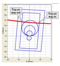
The first case for early tripping or trip on the way in resulted in tripping at 51.222 cycles from the start of the test, before the swing slip angle reaches 180° as shown in Fig. 31.
