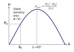
Fig. 2. The Power Angle Curve
