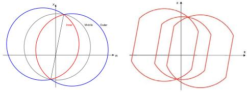
Fig. 13 Triple Characteristics for Power Swing Detection
