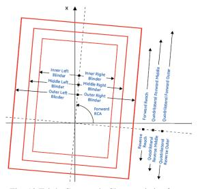
Fig. 12 Triple Concentric Characteristics for PSB and OST functions
