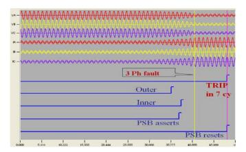
Fig. 37 Power Swing and Fault in Zone 1 Inside Inner Set of Blinders
