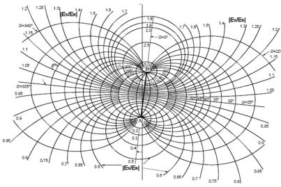
Fig.7. Impedance Trajectories for Various Ratios of  $|E_S/E_R|$
