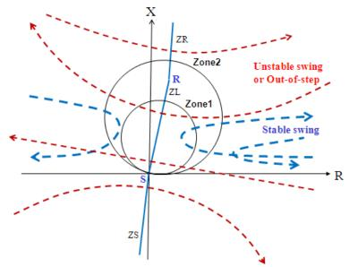
Fig. 8 Impedance Trajectories Seen By a Distance Relay at Bus S during Power Swings
