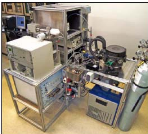
The NREL hydrogen safety sensor test facility (Robert Burgess/NREL) PIX 18240
