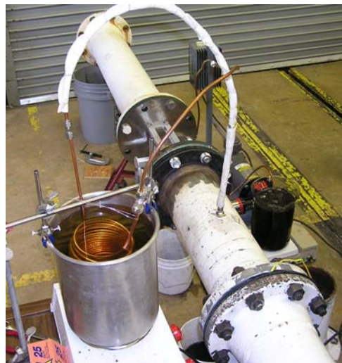
Figure 31. Heated Dirt/Water Injection Setup
