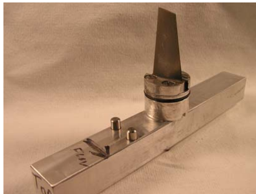
Figure 11. Blade Mounting Fixture with Blade Installed
