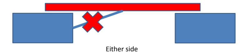
Ends rests freely on supports. No gluing, taping, affixing, Fastening, holding, weighting
