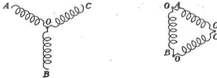
FIG. 4.—Coils of Fig. 1 connected together and placed on an alternator in order OA , OC , and OB .
