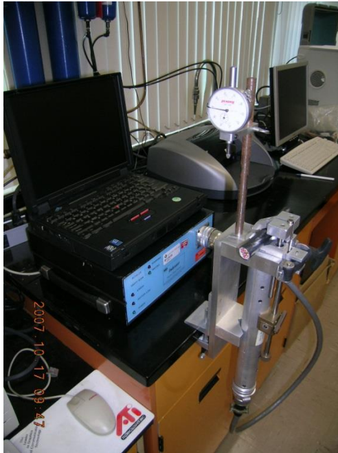
The Indenter Tool as used in the lab
