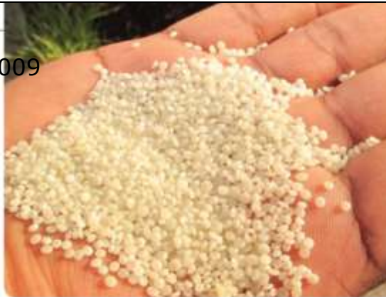
WASTEWATER WONDER: Ostara's Crystal Green, a slow-release fertilizer, incorporates phosphorus retrieved from sewage streams.
