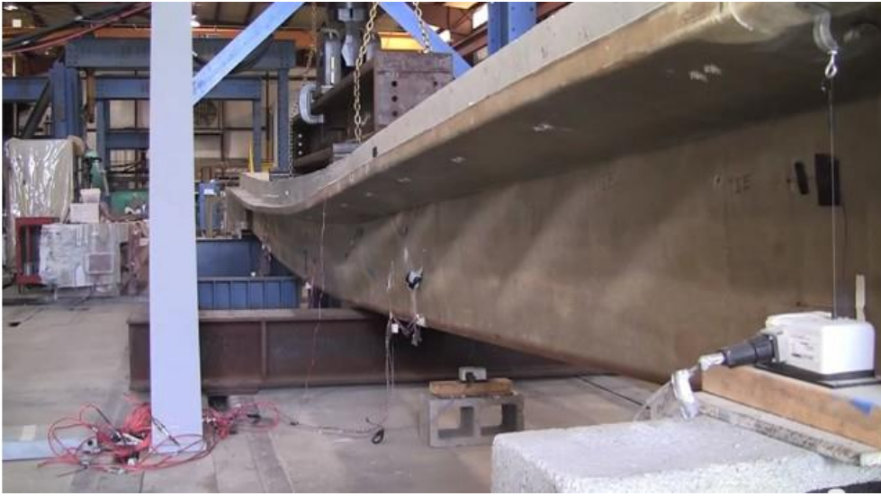
Figure 2. Tension field action in HCB (photo courtesy of Virginia Tech).
