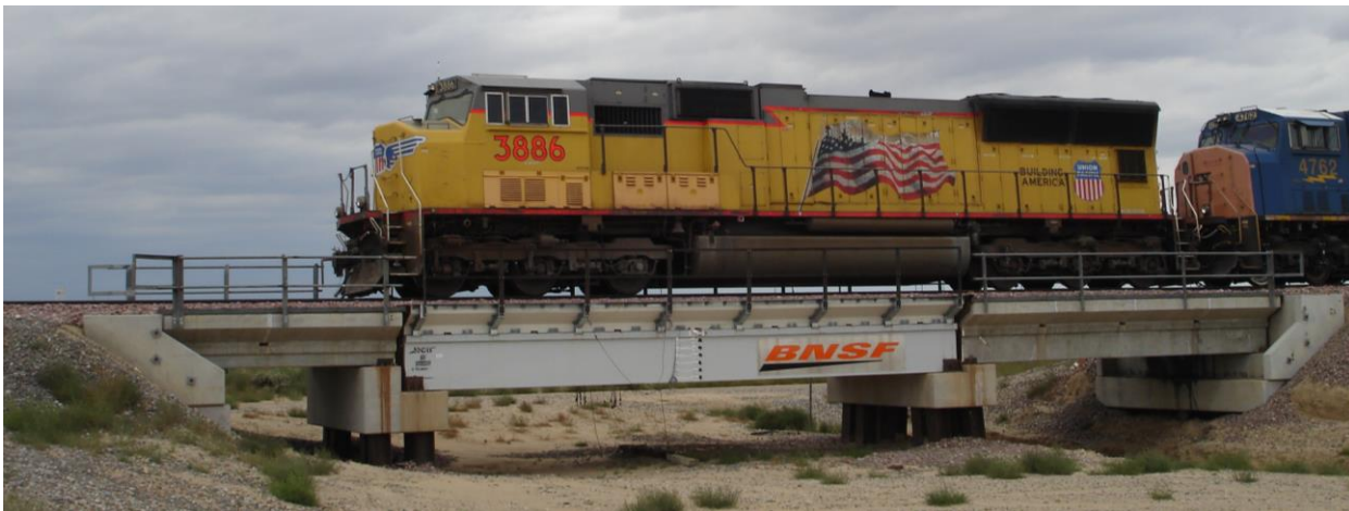
Figure 5. Test train crossing 42-foot HCB span at TTCI Pueblo, CO, test facility
