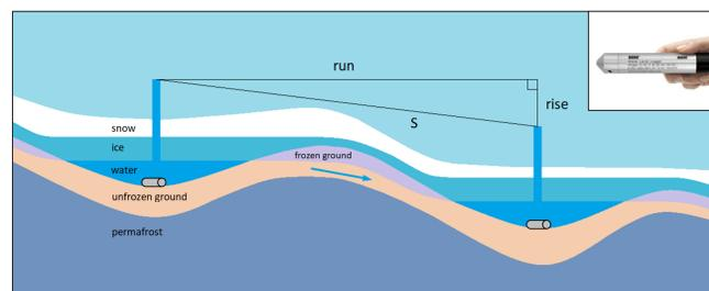
Figure 7: Winter stream channel longitudinal profile showing gradient  $S$  in hydrostatic water level. Blue columns are exaggerated to represent hydrostatic water level, which can be measured by submersible pressure recorders (inset).
