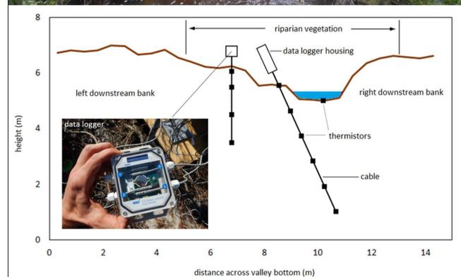
Figure 6: Instrumentation at Havikpak Creek intended to show the cross-sectional ground temperature field beneath the creek.
