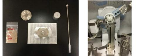
quantitative X-ray diffraction (qXRD) (quartz, K-feldspar, plagioclase, dolomite, phyllosilicates)
