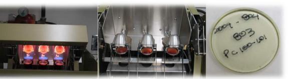
energy dispersive X-ray fluorescence (EDXRF) (Al, Si, K, Mg, Ca, Ti, Mn, Fe, P, Sr, V, Cr, Zn, Zr)
