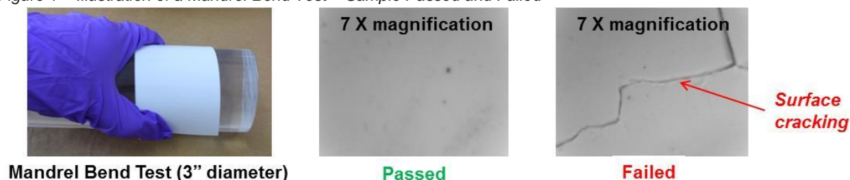
Figure 1 – Illustration of a Mandrel Bend Test – Sample Passed and Failed
