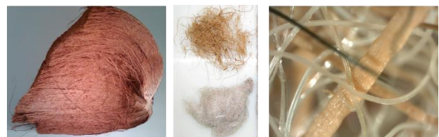
Figure 6 Inside of coconut husk, tufts of coir fiber from husk and PP binder fiber, seen in scanning electron microscope (SEM) after being carded and needle punched.
