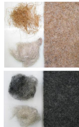
Figure 5. Comparison of tufts of coir (fiber) and propylene fiber (top) and tufts of PET and PE binder fiber (bottom). These are carded and needle punched for felt used to compression mold into trim parts.
