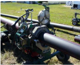
Typical HDPE Butt weld field fabrication machine
