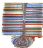
Good weld cross section
