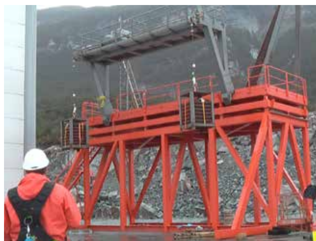
Load testing onshore R-002 cantilever davit
