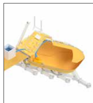
Full system test of deluge system with boat still in the davit
