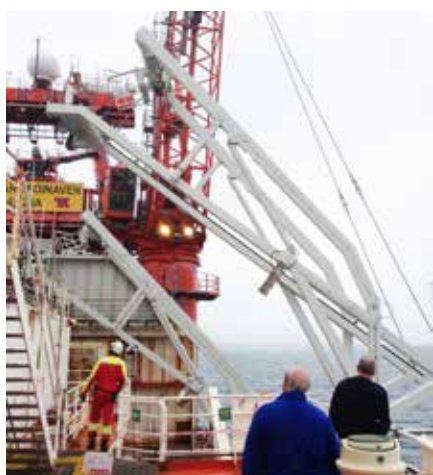
New free-fall davit, welded in place and connected
