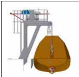
Lifeboat safely suspended in the davit to allow full maintenance
