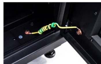
Earth straps on front and rear doors
