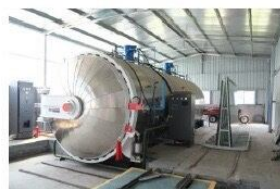
Pressure kettle, high pressure and temperature add, keeping and release. Pressure more than 12kg and temperature more than 120°C
