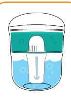
Tap water is gravity fed through a replaceable filter allowing for a constant and conveinient supply of fresh filtered water.
