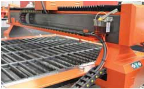
Industrial quality gantry, bellows and tracks.
