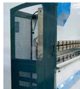
Premium fixed side and rear guarding (interlocked)
