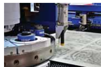
Optional Turret Upgrade to 40 station with 2 auto index (D)
