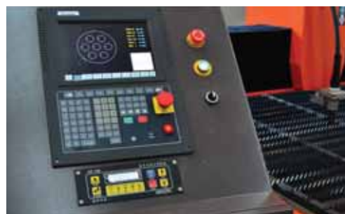
Starfire CNC System with 10 inch colour LCD display and real-time cutting path
