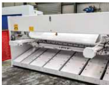
Quality backgauge with pneumatic sheet support system
