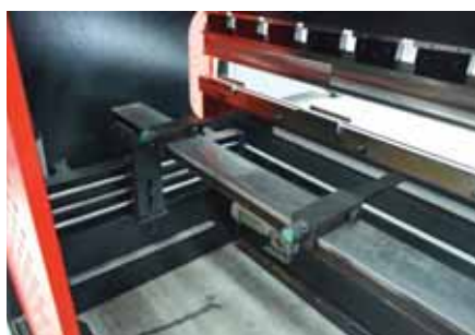
Servo Driven Ballscrew Backgauge
