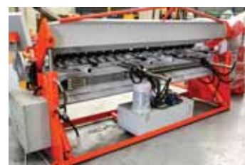
Compact hydraulic power pack and full backgauge
