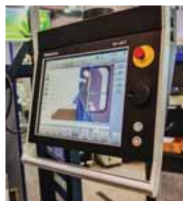
DA66T (Touch) controller with offline software available (2D and 3D optional)
