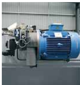
Hoerbiger hydraulics from Germany (complete assembly)
