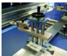
Easy adjust micro backgauge fingers, free moving on linear guides
