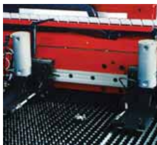
Heavy duty automatic clamping system
