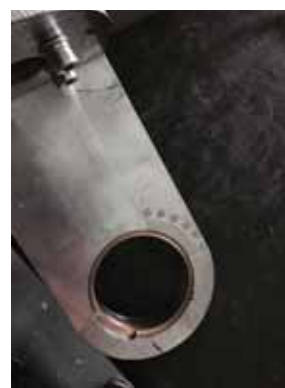
Fine adjustment of the cutting head angle to allow for tapering of the jet
