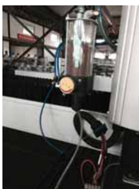
Fine Adjust of Garnet Delivery
