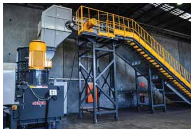
Genox Z1500 shredder as part of a toner recycling line
