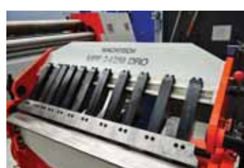
Extra long clamps. 60 x 75mm solid steel
