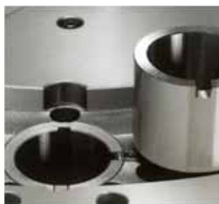
Hardened die bush. Amada style thick turret
