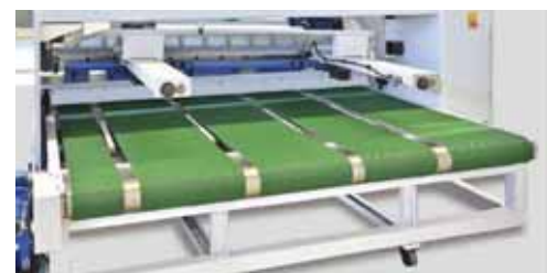
Rear takeout device with PU conveyor
