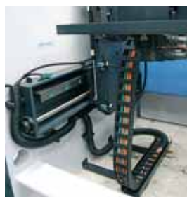
All linear rails and slides are premium THK units
