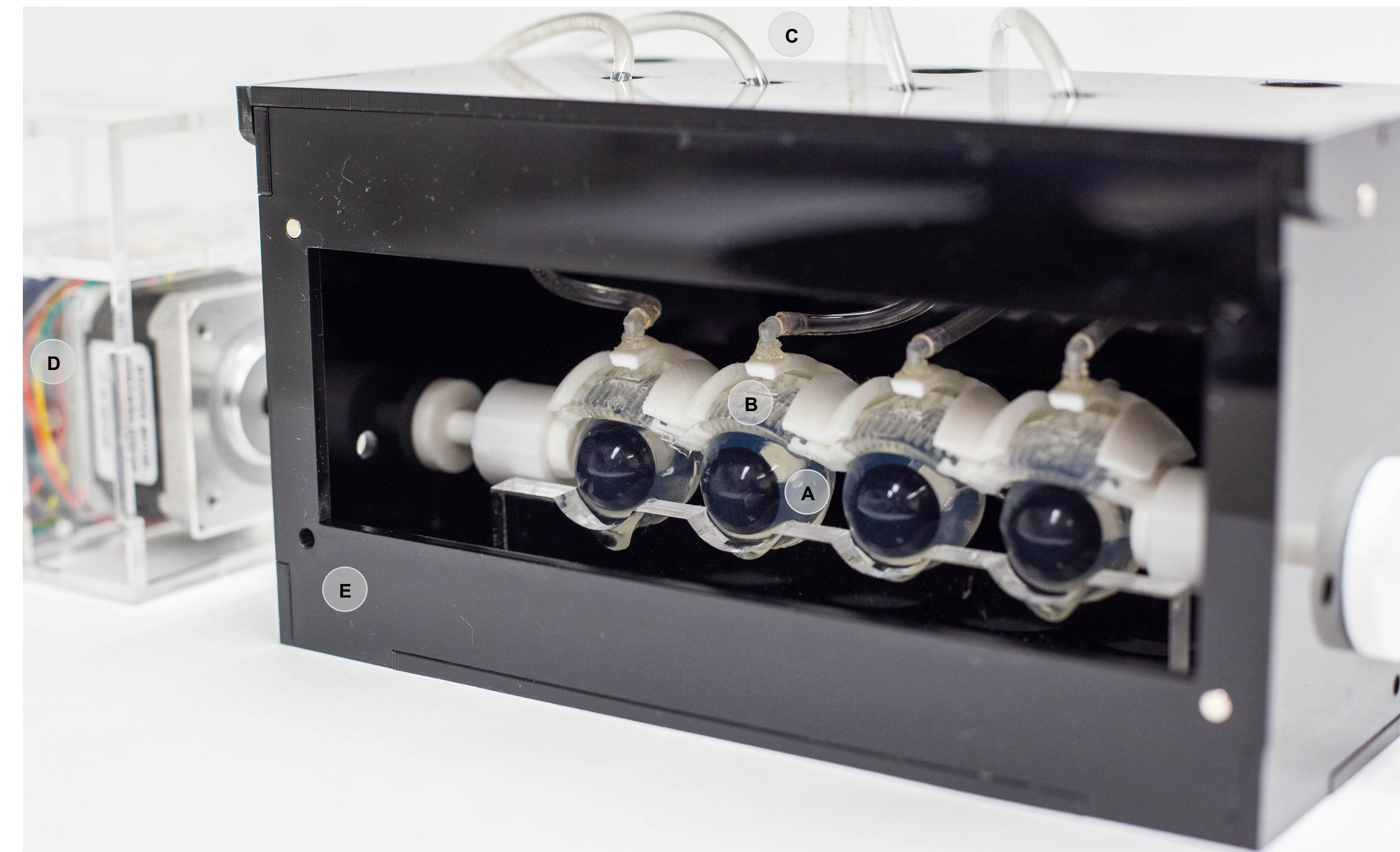
Figure 1. In vitro eye model showing the A eyeball, B eyelid, C tubing, D motor and E casing.
