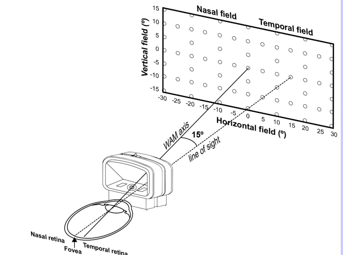
Figure 2 Experimental setup to measure the RPRE
