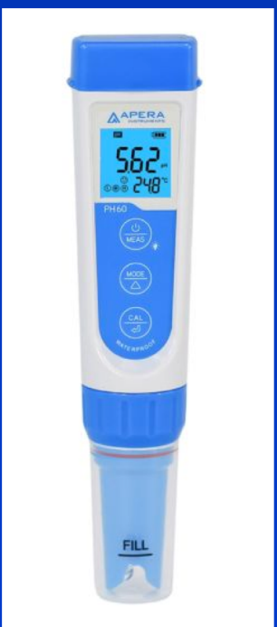
Figure 1: Picture of the Apera pH meter used in this study
