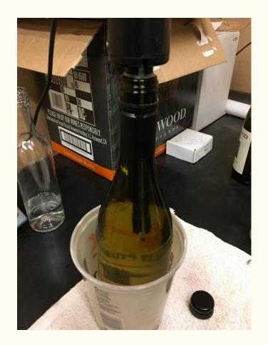
• Torque test – screw cap
