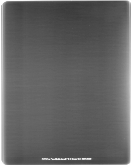
Figure 3 Level 7F low Mottle VCS (minimum accept)
