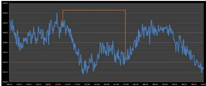
Figure 7 Step height model for evaluating flow mottle
