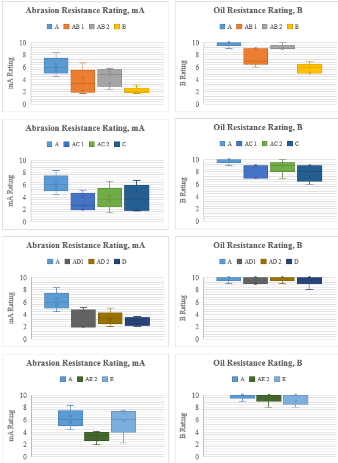
Figure 7. Shaker Table Abrasion Test results for ionomers and their blends
