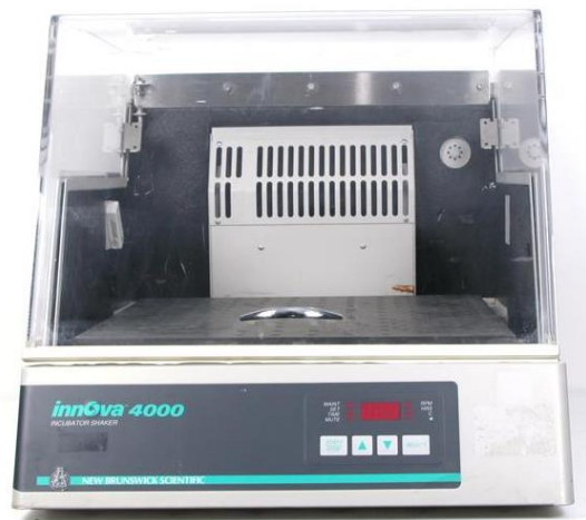
Figure 2. The shaker used for this experiment [5].
