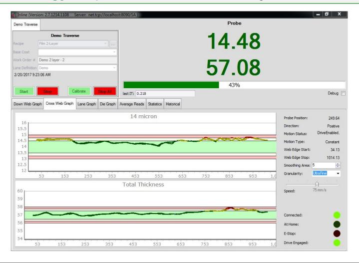
Dual line configuration for sequential measurement of two coating layers
