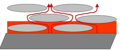
Nanoparticle inkjet - ~500 nm thick Micron flake screen print - ~5-30 microns thick
