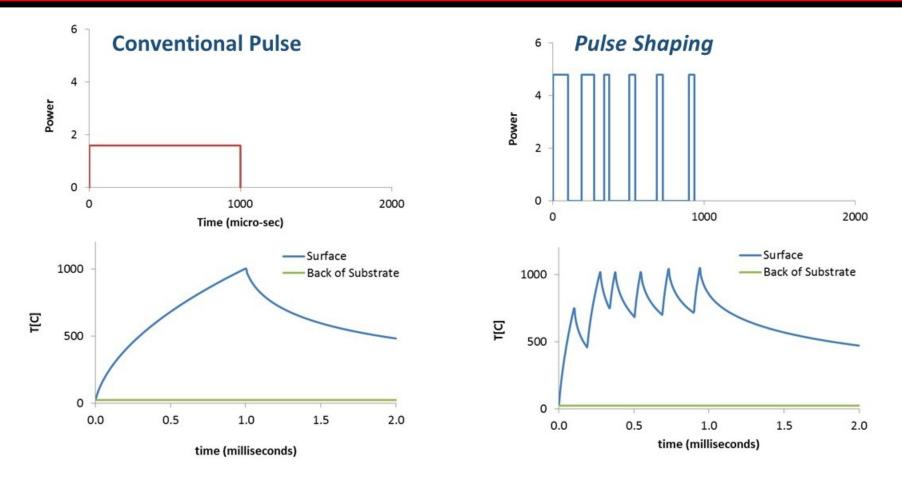
Pulse Shaping: Multiple pulses acting within the thermal equilibrium time of the material.
