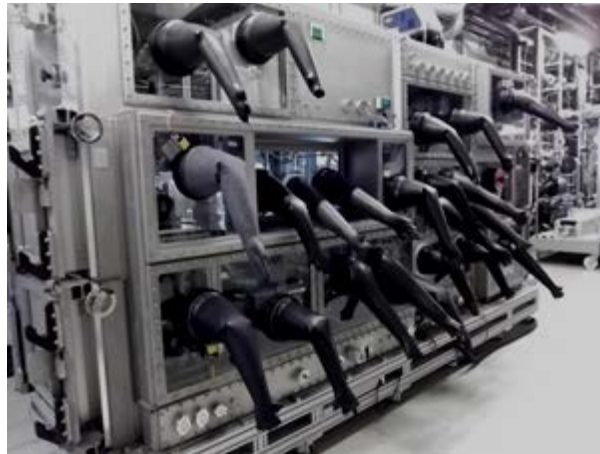
Figure 3: Photograph of R2R lamination system which is encased in an inert box at Fraunhofer FEP. The butyl gloves allows still high flexibility in process variations under R&D conditions.
