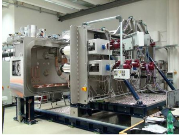
Figure 2: A photograph of the roll-to-roll OLED vacuum coater with 14 organic linear sources, plasma source for pre-treatments, 2 metal evaporators for the electrode deposition and magnetron sputter system for pre-encapsulation with metal oxide.
