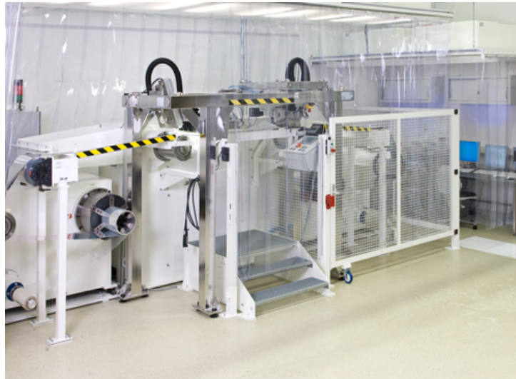
Figure 4: Roll-to-Roll optical inspection system encased in a clean room carbine ISO6 to minimize particle contamination during inspection process.
