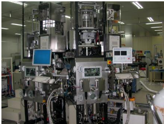
200 mm System: Glass substrates, metal and polymer web, flexible glass up to 200 x 200 mm 2
