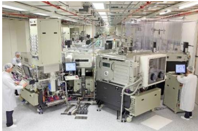
Gen2 Line: Glass substrates 370 x 470 mm 2
