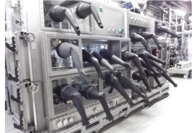
R2R printing and lamination unit (N 2 )
