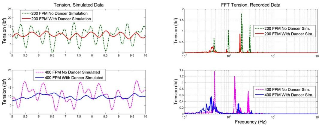
**Figure 10: Comparing Simulations of the Unwind Bump Disturbance without and with a Dancer. The 200FPM simulation shows an 84% reduction in magnitude of the Unwind 1-per-rev frequency. The 400FPM simulation shows a 61% reduction at the unwind 1-per-rev frequency.**
