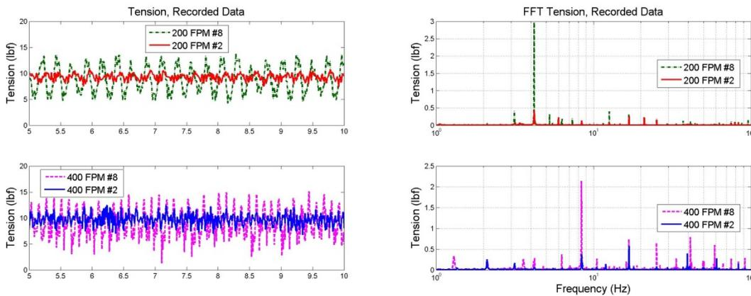
**Figure 7: Eccentric Idler Upstream (#2) of the Dancer vs. Downstream (#8), 200FPM (left, top), 400FPM (left, bottom), FFT of 200FPM (right, top), FFT 400FPM (right, bottom). The dancer has a large impact on the load cell sensed tension. It removes 83% of the magnitude at the 1-per-rev frequency at 200FPM and 80% at 400FPM.**
