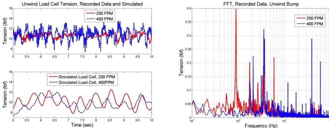
Figure 4: Unwind Roll Bump Disturbance, Recorded (left, top) Tension, Simulated (left, bottom), and Frequency Response (right). The Unwind 1-per-rev is a driver, but span natural frequencies show up.
