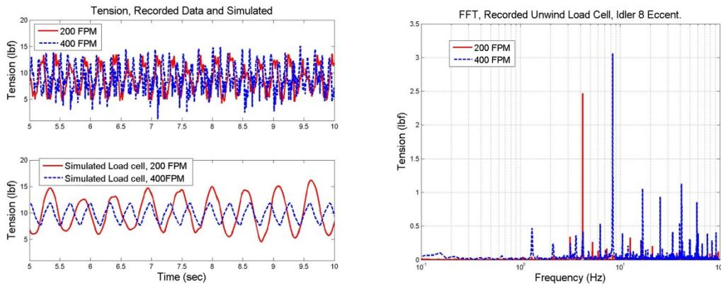
**Figure 6: Eccentric Idler Downstream of the Dancer, Recorded Tension (left, top), Simulated Tension (left, bottom), FFT (right). Recorded data show a ~10 lbf peak-to-peak oscillation while the Simulation had near that for the 200FPM, but only about 5 lbf for the 400FPM case.**
