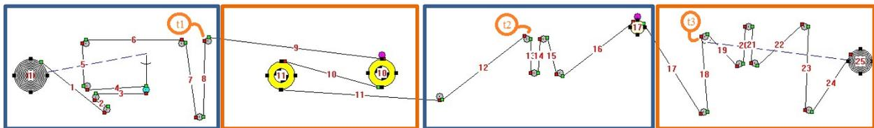
Figure 1: System schematic diagram with 4 sections from left to right: the unwind, the S-wrap, the pull roll, and the Rewind sections. T1-3 are the locations of load cells which are used for measurement and/or control.
