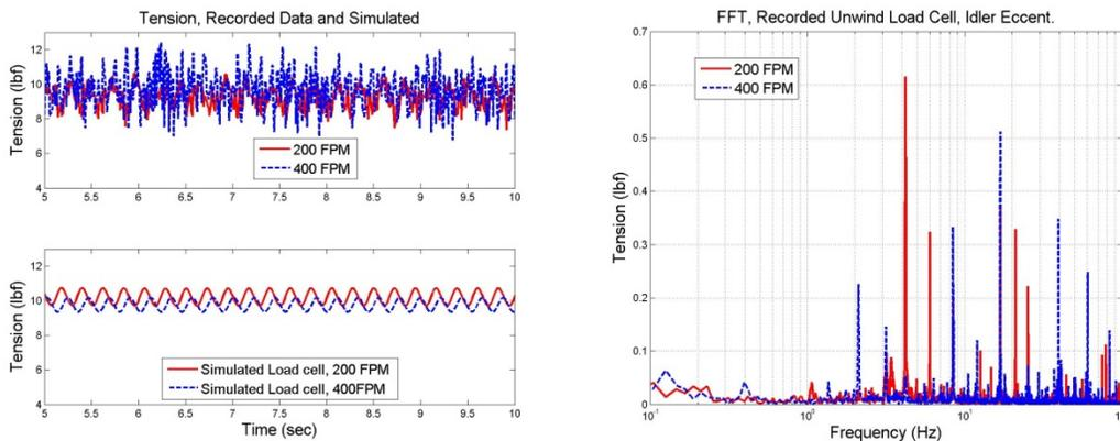
Figure 5: Idler #2 Eccentricity, Recorded Tension for 200 and 400 FPM process speeds (left, top), Simulated Tensions for the same (left, bottom), and FFT of Recorded Data (right). The idler frequency is the first large magnitude for both speeds.
