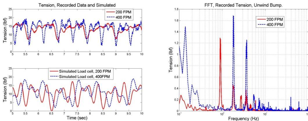
**Figure 8: Unwind Bump Disturbance with No Dancer, Recorded Tension (left, top), Simulated Tension (left, bottom), FFT (right). The unwind 1-per-rev frequency (0.91Hz for 200FPM and 1.8 Hz for 400FPM) is clearly present as are several harmonics. The time domain data shows a slow oscillation at 400 FPM that shows up as low frequency peaks in the FFT.**
