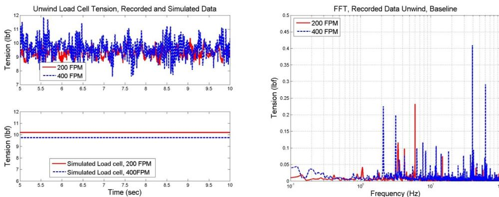
**Figure 3: Baseline Tension, Recorded Tension (left, top), Simulated Tension (left, bottom), FFT (right). The simulation curves are offset artificially by adjusting the input force to the dancer in order to show the general character of both.**
