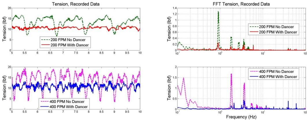
**Figure 9: Comparing the Unwind Bump Disturbance without and with a Dancer. Without a dancer, the oscillations are much larger and sharper (note the zoomed in time scale). The dancer removes 83% of the 1-per-rev frequency magnitude at 200FPM and 82% at 400FPM.**
