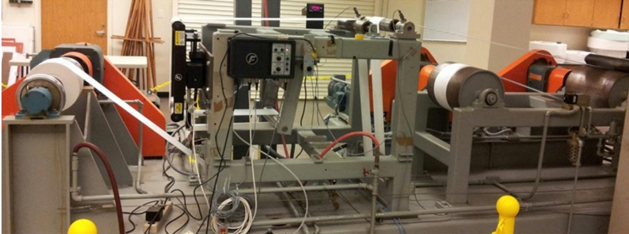
Figure 2: Unwind section of Euclid Web Line at Oklahoma State University. The unwind roll is at the left and the forward process direction is to the right, ending with the S-wrap (large rollers on the right).
