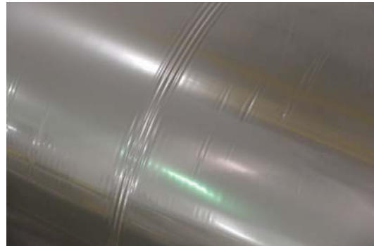
Figure 2 – Corrugation Caused by A High-Low-Medium Caliper
