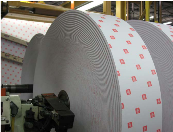
Figure 4 – Oscillation Offsets in a Wound Roll
