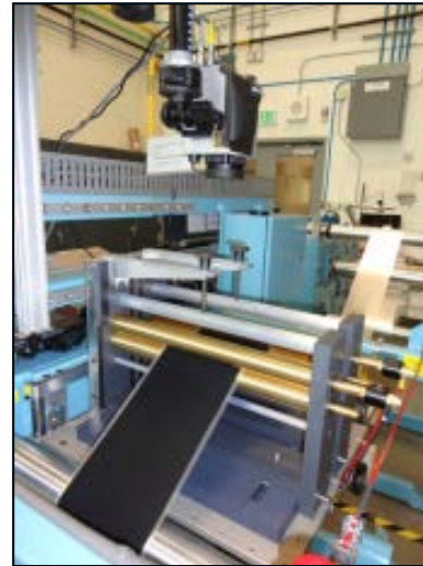
Infrared imaging of electrode and cell defects
