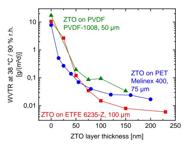
reactive dual magnetron sputtering zinc-tin-oxide (ZTO)
