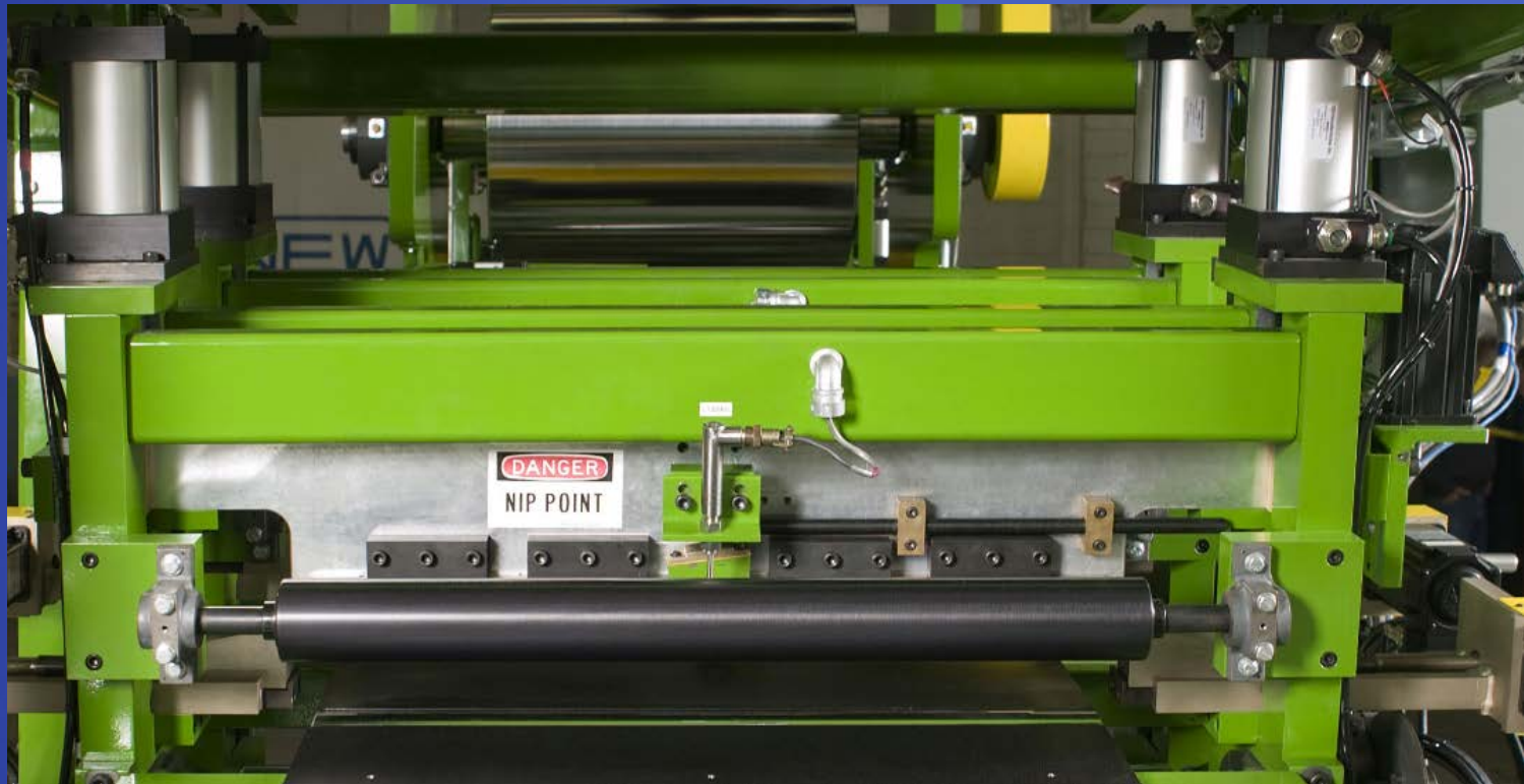
Knife Coater with Automatic Blade Bending
