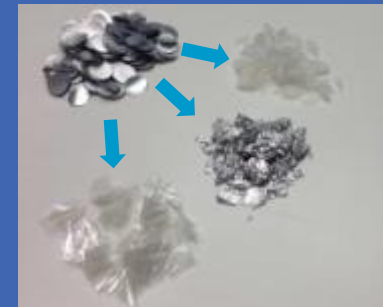
Typical LD-PE/Alu/PET pouch-material after delamination
