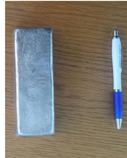
Aluminium ingot produced from the flakes
