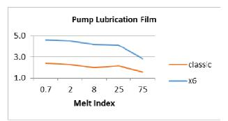
Figure 10: In the 20 tph PP plant, the x6 class pump operates with approximately 2 times the lubrication film thickness of a classic pump.
