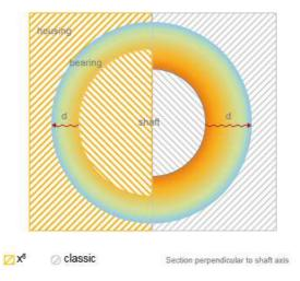
Figure 2: Modified bearing design reduces bearing temperature and effectively increases the pump speed limit to make higher flow rates possible.
