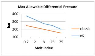
Figure 11: In the 20 tph PP plant, the x6 class pump gives the user the possibility to operate with 1.5x higher differential pressure than a classic pump.
