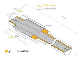
Figure 1: The larger shaft journal diameter of the x6 class pump makes it possible to have longer gear teeth for higher specific volume, without sacrificing the pump's pressure-building capability.
