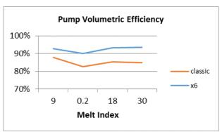
Figure 4: In the 60 tph HDPE plant, a classic pump operates at 85% volumetric efficiency, while the x6 class pump operates at 92% volumetric efficiency.
