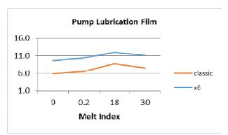
Figure 7: In the 60 tph HDPE plant, the x6 class pump operates with approximately 1.5 times the lubrication film thickness of a classic pump.
