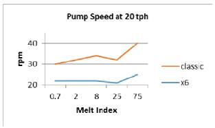
Figure 9: In the 20 tph PP plant, a classic pump operates at 34 rpm, while an x6 class pump of the same size operates at 22 rpm.
