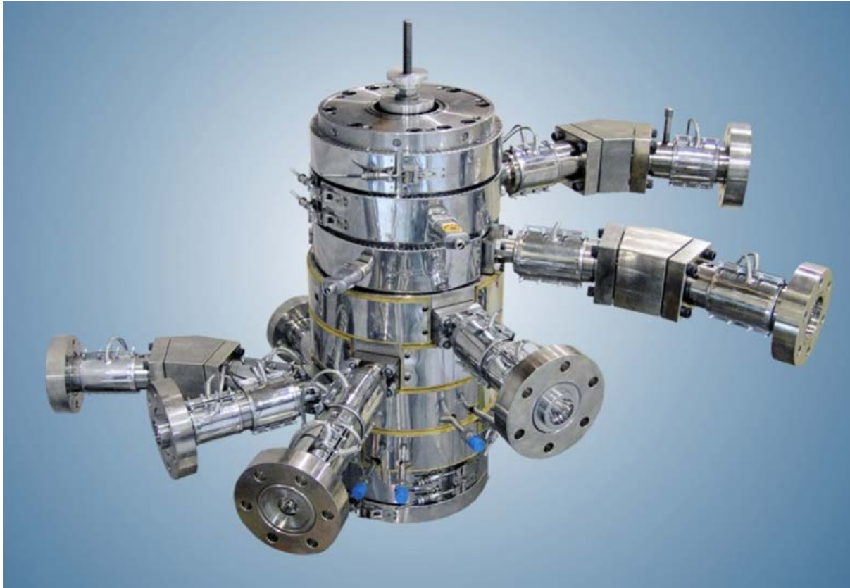
7-Layer Taper Pack Macro Engineering Coextrusion Die for Heat Shrinkable Biax Film, Courtesy Macro Engineering
