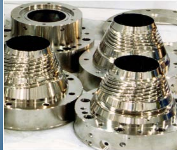
7-Layer Taper Pack Macro Engineering Coextrusion Die for Heat Shrinkable Biax Film, Courtesy Macro Engineering
