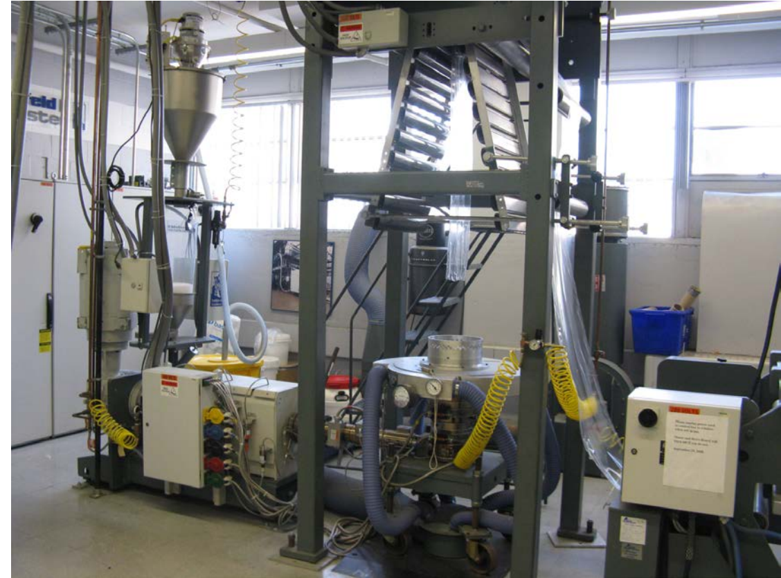
UMASS-Lowell Plastics Engineering Department Mono-Layer Blown Film Lab Photo by Tom Bezigian
