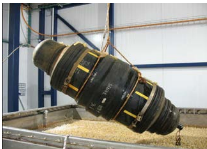
Figure 12. 630SDR17 Gas Pipe and Electrofusion Coupler During Hydrostatic Pressure Testing
