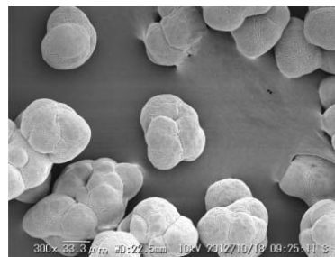
Figure 3. SEM image of polymer obtained by using rac -Et(Ind) 2 ZrCl 2 supported Solid MAO catalyst shown in table 1 (x300).
