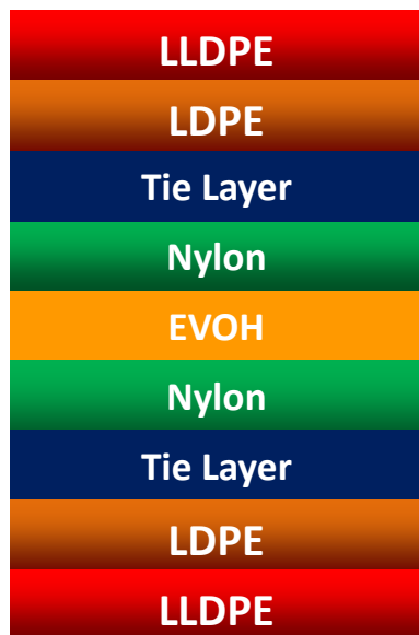
Fig. 3D 9-layer rigid, high barrier structure using cost/performance optimized PE resins
