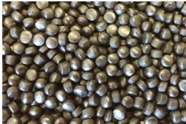
Figure 4. PP pellets from upgraded ASR after compounding flakes with small amounts of additives
