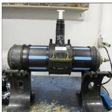
Figure 13. 110SDR17 Water Pipe and Tapping Saddle Electrofusion Assembly Ready For Product Testing
