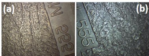
Figure 3. (a) Grain pattern of the tool used for producing skin, (b) grain pattern of the polyolefin skin produced.
